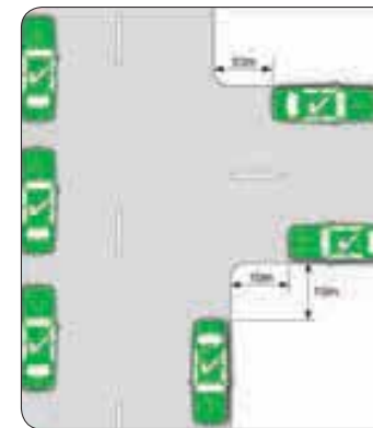
Example 52 Measurement of distance — T-intersection without traffic lights.
